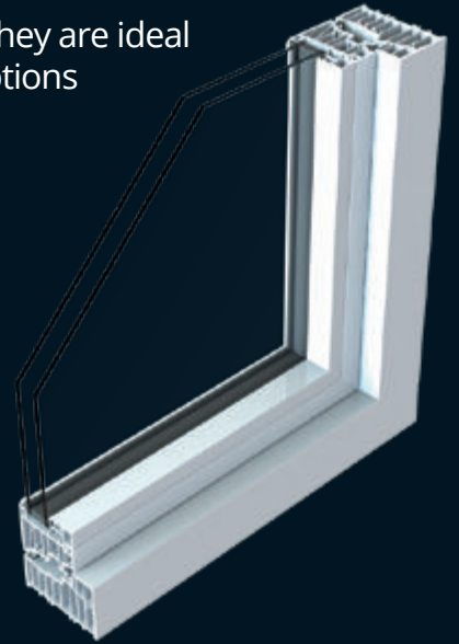
100mm 9 chambered energy efficient profile achieving 0.79 W/m 2 k U-Value for 28mm double glazing or 44mm triple glazing
